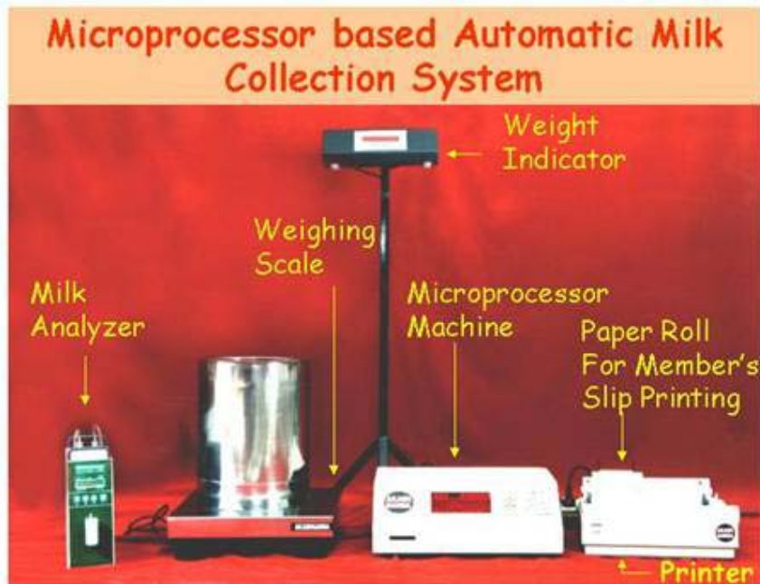
Microprocessor-Based Automatic Milk Collection System (AMCS)
