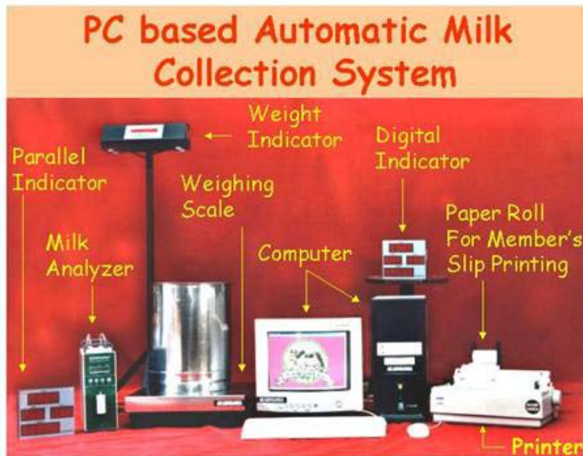
PC-based Automatic Milk Collection System (AMCS)
