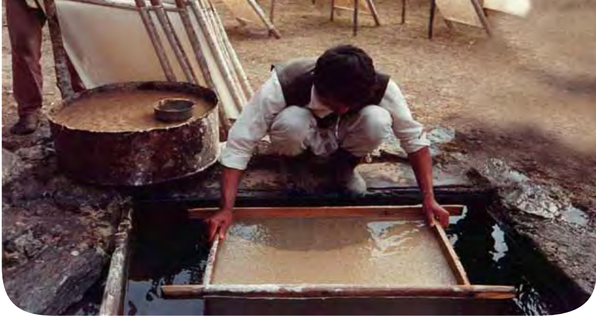
Sizing paper pulp in a wooden frame
